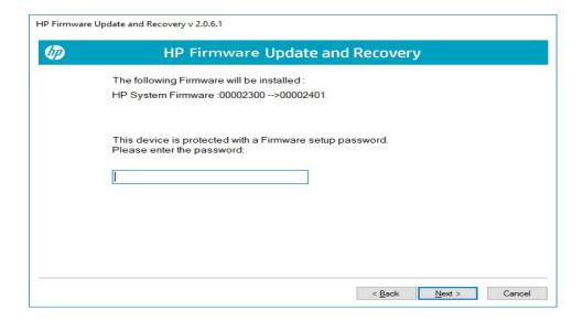
both displayed. The user is notified that the firmware will be overwritten. Enter the firmware setup password into the password field if BIOS has set an administrator password, then select Next.
