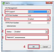
8. Press the Apply button at the bottom of the main BACS 4 screen to apply the settings. A dialog box displays a note that the network connection will be lost as the settings are saved. This is normal.
