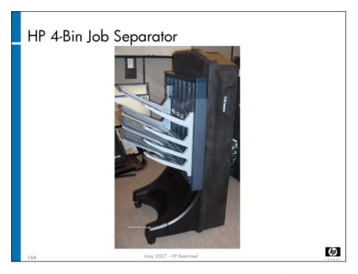
The HP 4-Bin Job Separator is an optional accessory, and can be used with the MFP instead of the single output bin or the HP Multifunction Finisher. It is a scaled-down version of the multifunction finisher, without the staplers or the accumulator.
