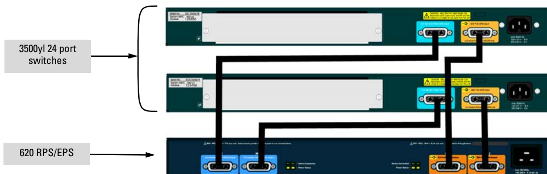
Figure 3-2. Example of two 3500yl-24G-PWR Switches connecting to a ProCurve 620 External and Redundant Power Supply (J8696A)
