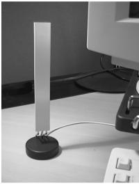
Use the Range Extender Antenna when the integrated antenna of the HP Wireless AP Card 150wl is concealed or shielded, for example:
