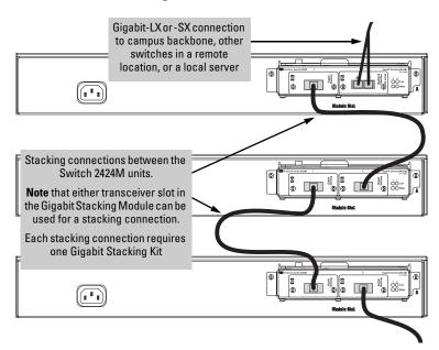
**Note:** If the stack is connected to any other switches, the number of switches in the stack must be reduced so that the total number of interconnected switches is at most seven.
