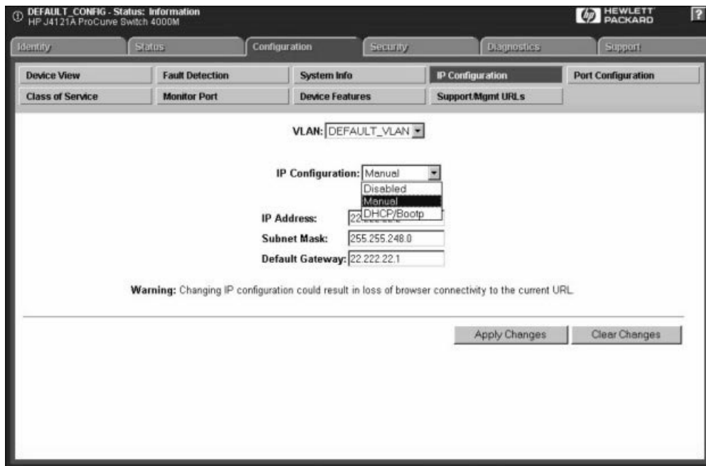
Figure 7-3. Switch IP Configuration
