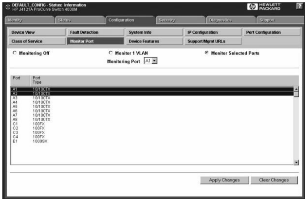
Figure 7-5. Selecting a Monitoring Port on a Switch
