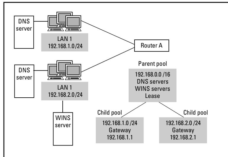
Figure 13-3. Example DHCP Pool Configuration
