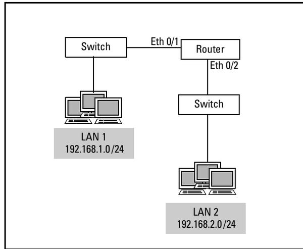
**Figure 13-2. ProCurve Secure Router DHCP Server**
