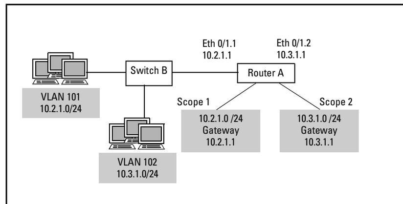
**Figure 13-4. DHCP Scopes with VLANs**
