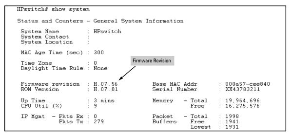
Figure 3. Example of Using the CLI 'show system' Command to Verify the Software Revision
