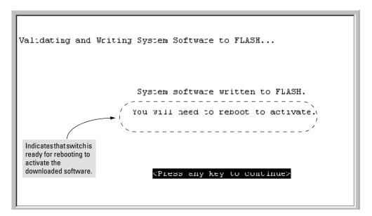
Figure 2. Message Indicating the Switch Is Ready To Activate the Downloaded Software
