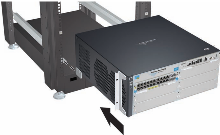
Figure 4. Notches in Bracket Being Installed
