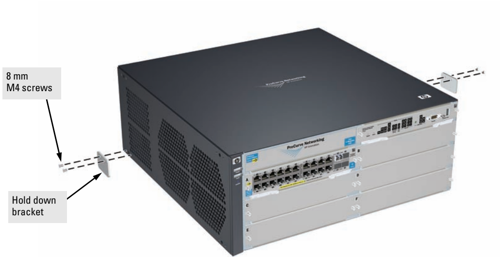
Figure 2. Attaching Hold-Down Bracket to a Series 5400zl Switch
