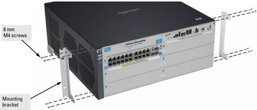
Figure 3. Attaching Brackets to the 5400zl Switch
