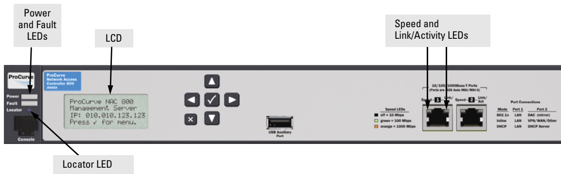
Figure 1. ProCurve Network Access Controller 800 LEDs and LCD
