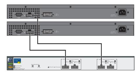
In this example each switch receives 408 watts of PoE power. Each switch is connected to one port of each pair. If the two switches were connected to both ports of a pair, both ports of pair A for example, then each switch receives 204 watts. See the following example.
