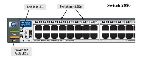
When the switch is powered on, it performs its diagnostic self test. Self test takes approximately 50 seconds to complete.
