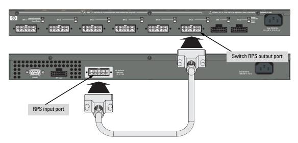
The following illustration shows an example of connectivity between an RPS/EPS device and six switch devices as a redundant AC power supply.
