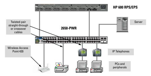
The Switch 2600-PWR Series devices are also designed to be used as desktop switches to which end nodes, printers and other peripherals, and servers are directly connected, as shown in the above illustration. Except now these switches can supply PoE power to end devices such as IP telephones and wireless access points (WAP).
