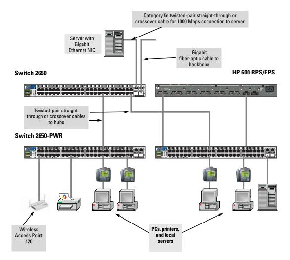
As shown in the illustration above, the IP telephones have been inserted in between the Switch 2650-PWR and the PCs, and a WAP has been connected to the Switch 2650-PWR. Both the telephones and WAP will receive PoE power from the Switch 2650-PWR. Only devices directly connected to the PWR switches can receive PoE power if they are 802.3af compliant. Devices connected to a non-PWR segment switch cannot receive PoE power.
