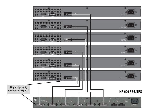
The HP 600 RPS/EPS can provide backup power for up to six switches. The HP 600 RPS/EPS can supply power to only one connected and failed switch at a time. In the illustration above, the switch connected to RPS port 1 has the highest priority and the switch connected to RPS port 6 has the lowest priority. When multiple switches fail, a switch connected to a higher priority port always receives power before a switch connected to a lower priority port.
