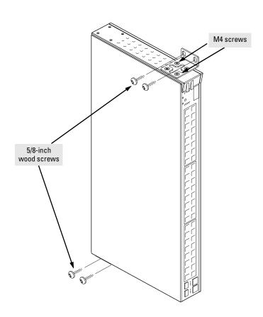
The brackets are attached on opposite corners to improve the stability of the switch on the wall.
