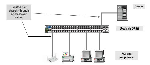
The Switch 2600 Series devices are designed to be used primarily as desktop switches to which end nodes, printers and other peripherals, and servers are directly connected, as shown in the above illustration. The end node devices are connected to the switch by straight-through or crossover twisted-pair cables. Either cable type can be used because of the "HP Auto-MDIX" and "IEEE Auto MDI/MDI-X" features on the Series 2600 Switches.
