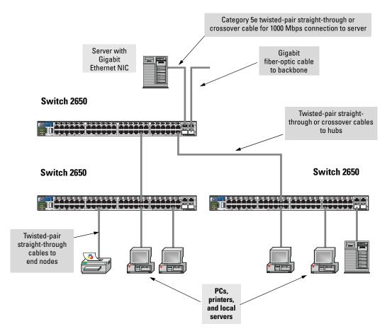
The Switch 2600 Series devices also work well as a segment switches. That is, with their high performance, they can be used for interconnecting network segments—simply connect the network devices that form those segments to the Switch 2600 Series devices.
