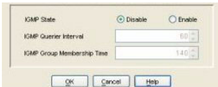
Figure 9-20. IGMP Setting for Routing Switches
