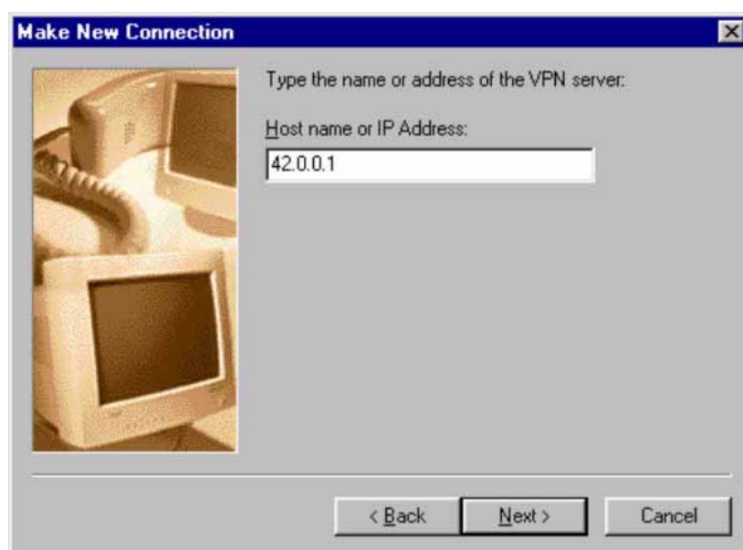
Figure 3-61. Make New Connection Window, VPN server address
