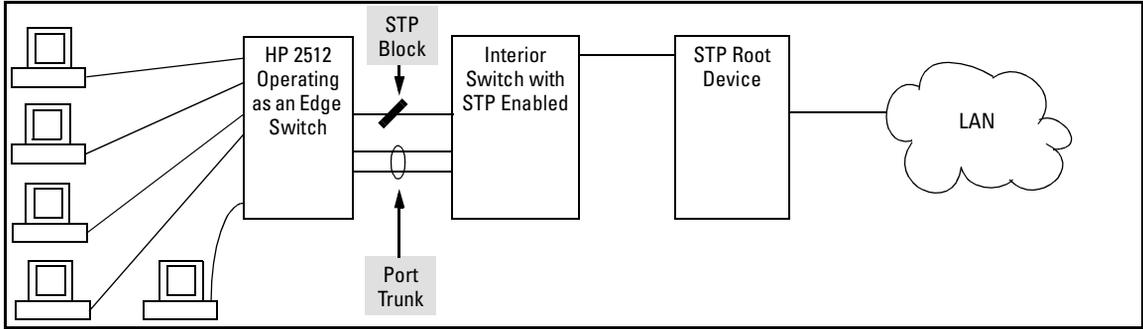
**Figure 8. Example Topology for the Listing Shown in Figure 9**
