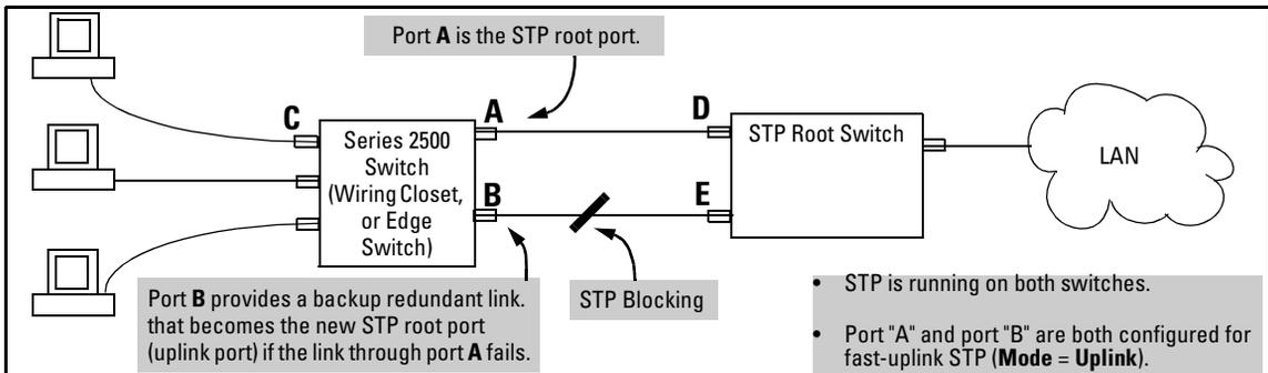
**Figure 1. Example of How To Implement Fast-Uplink STP**
