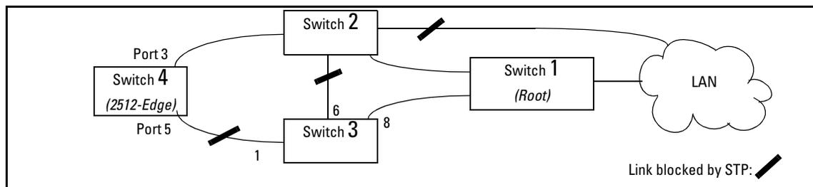
**Figure 2. Example of an Edge Switch in a Topology Configured for STP Fast Uplink**
