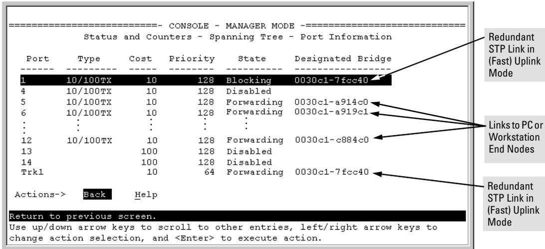
**Figure 7. Example of STP Port Status with Two Redundant STP Links**
