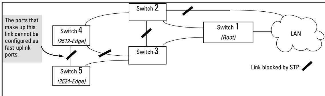
**Figure 3. Example of a Disallowed Connection Between Edge Switches**
