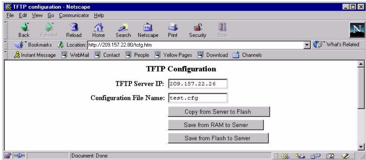
Figure 4.2 TFTP transfer screen for software configuration files
