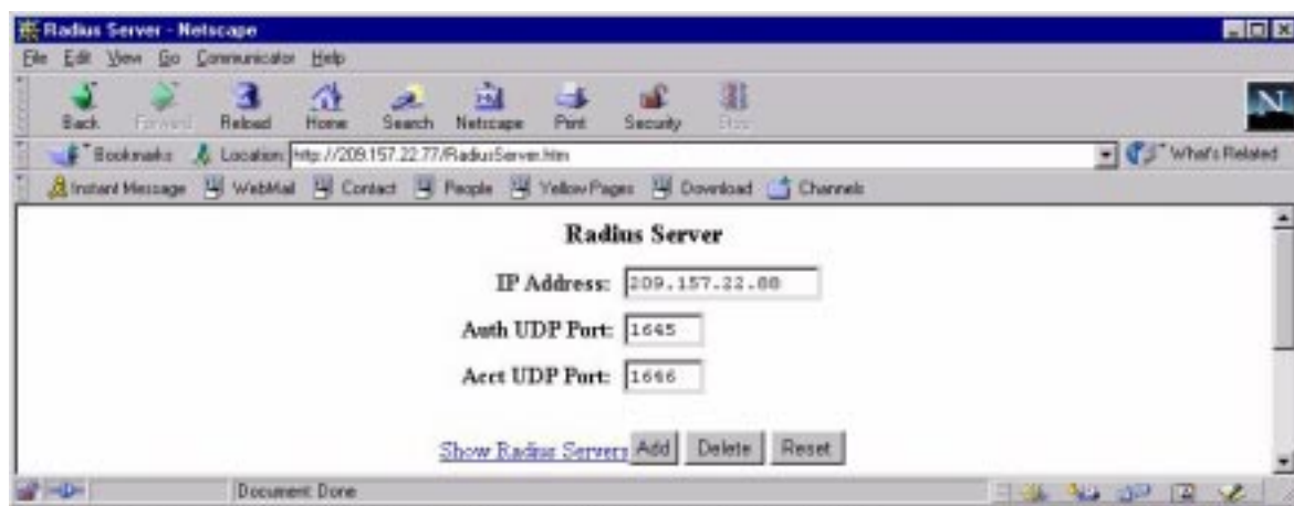
Figure 2.17 RADIUS Server panel
