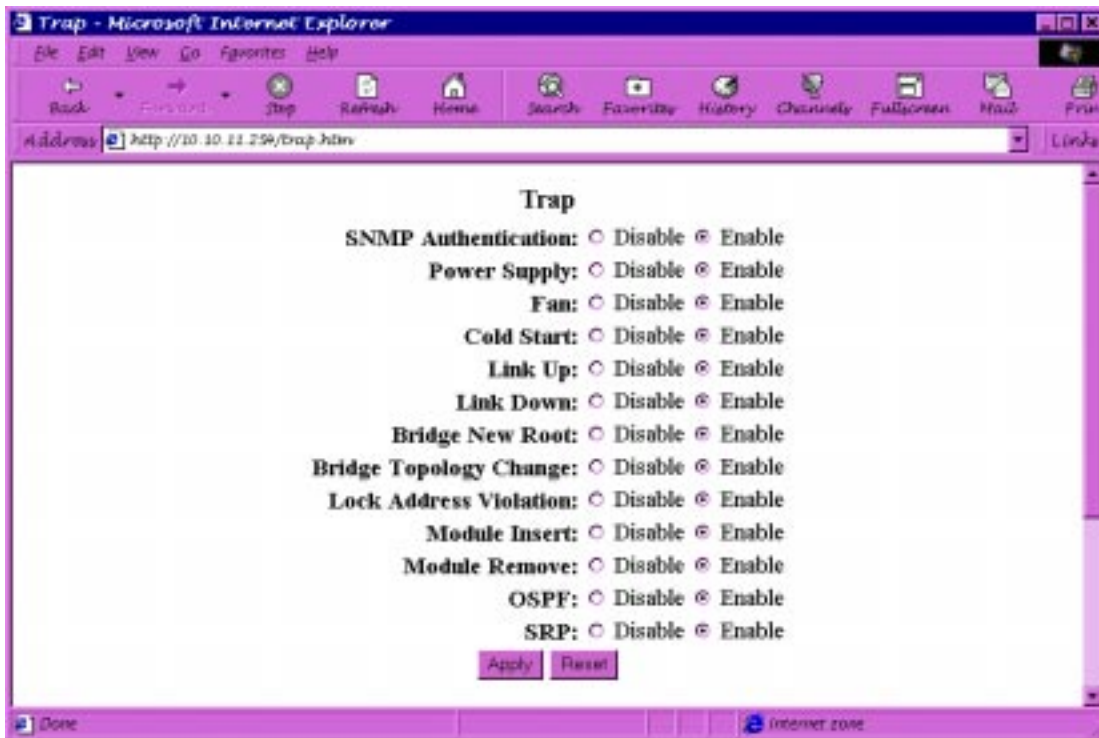
Figure 7.6 SNMP trap configuration panel for routing switches
