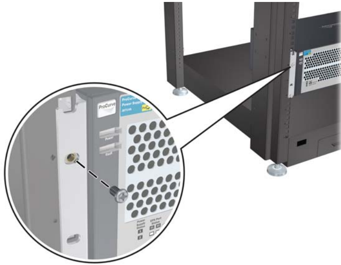
Figure 2-4. Installing top screws into bracket and rack
