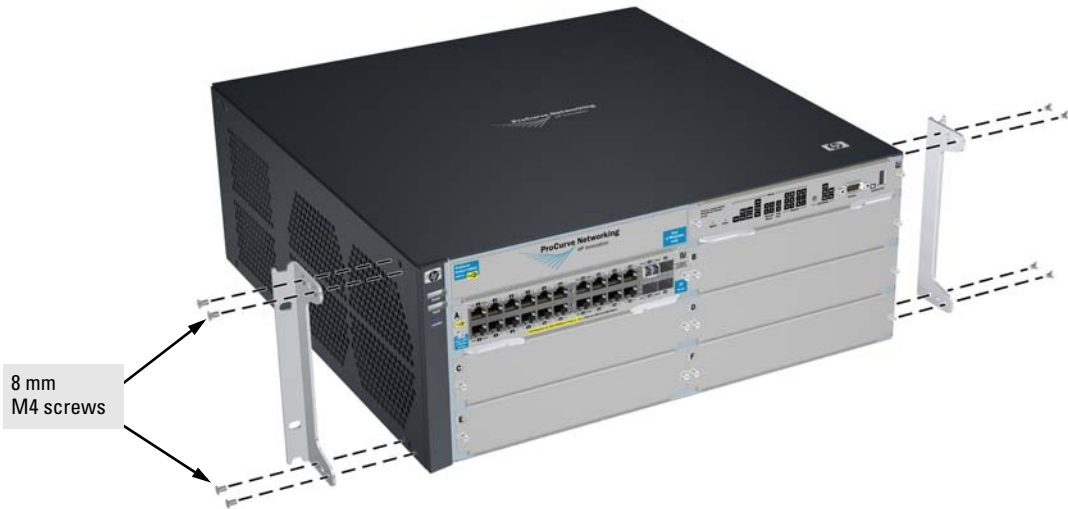
Figure 2-7. Attaching Brackets to the 5400zl Switch
