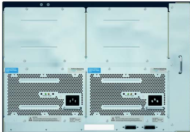
Figure 1-8. Back of a 5412zl Switch with two Power Supplies
