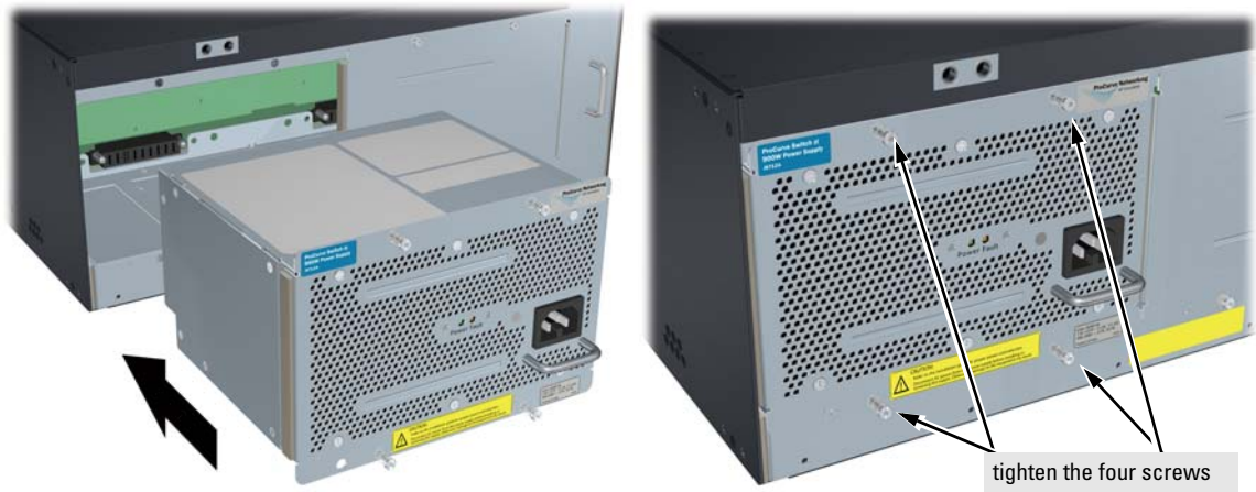
Figure 4-2. Power Supply Installation
