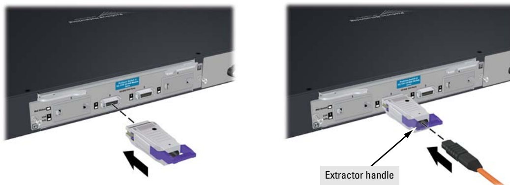
Figure 3. Installing an OMC
