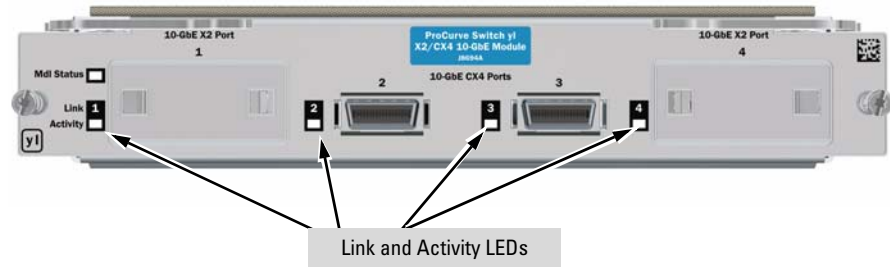
Figure 9. Example Link and Activity LEDs
